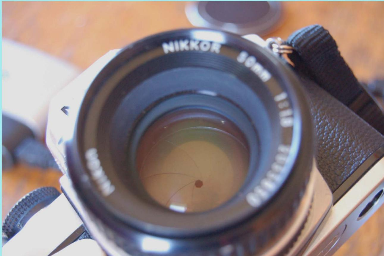
The higher the f-stop (smaller the aperture), the more of the photo will be in focus
